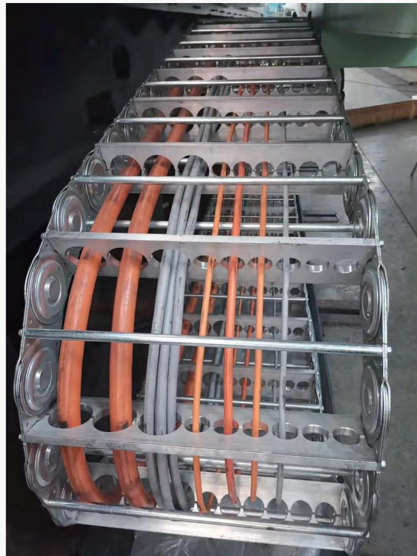
ZF-TL250 Series Steel energy chain for roll grinding machine
