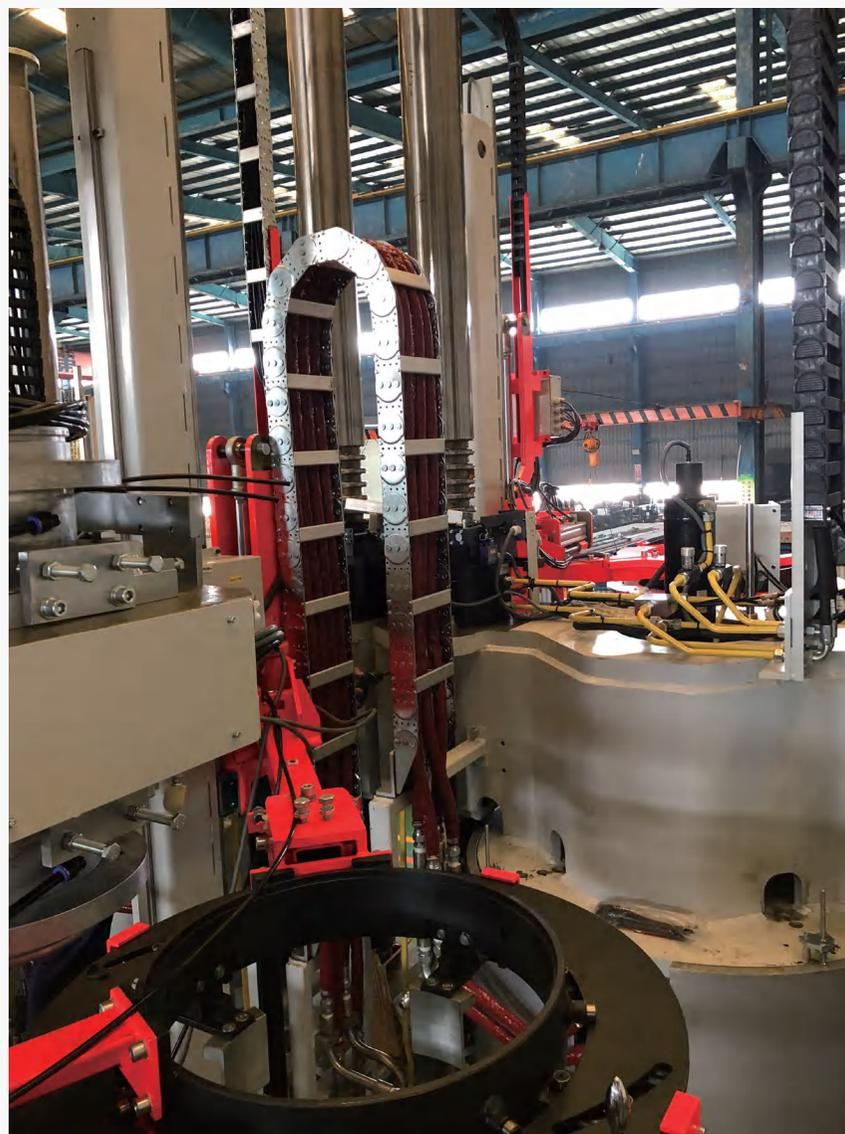
ZF-TL95 Series Steel energy chain used on tire curing presses
