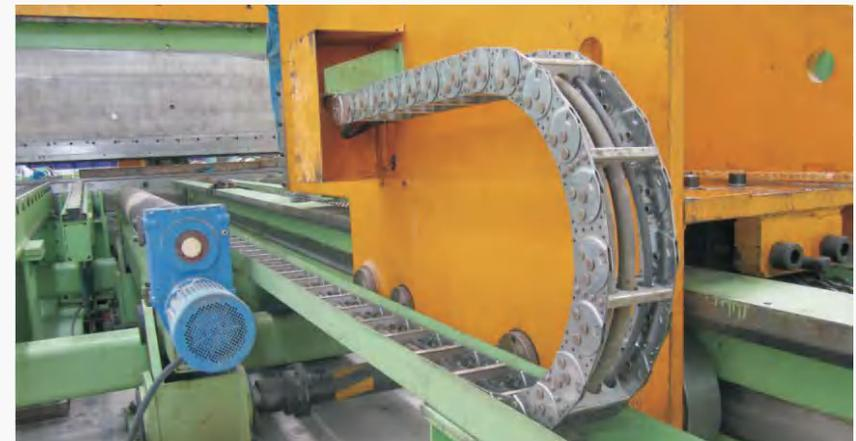
ZF-TL65 Series Steel energy chains are used on material handling equipment
