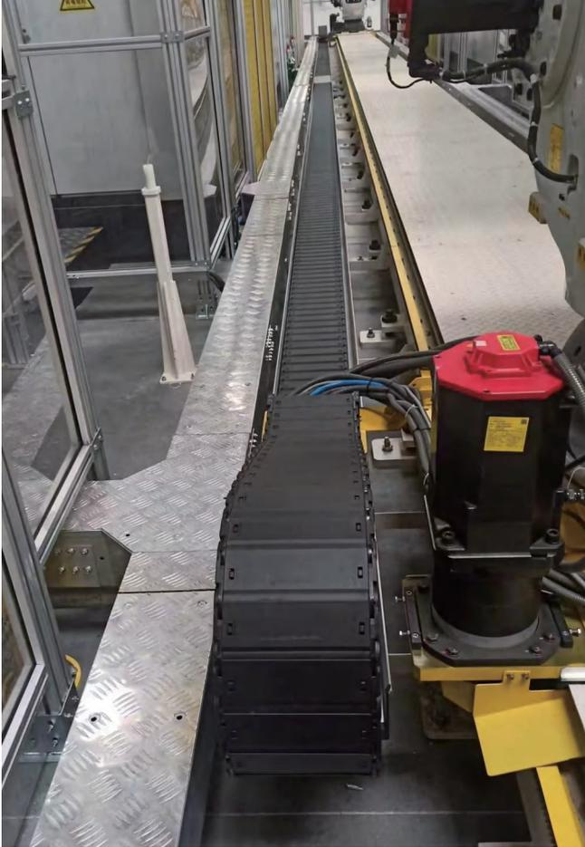
YFM5680.200.250.BK is used in the field of automated assembly line processing equipment.
