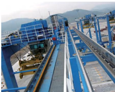
Guide through with glide-bar part: wear-resistant strip is made of high-density wear-resistant polymer material with low friction coefficient and low abrasion to the energy chain.
