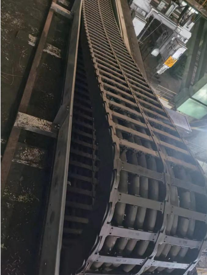
ZF8000.200/200.300.BK and guide groove accessories, used for long-distance heavy-duty sliding occasions in non-ferrous metallurgy.
