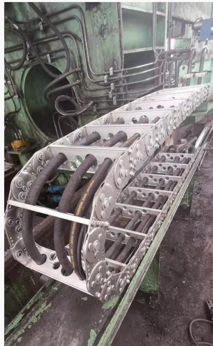
ZF-TL225 Series Steel energy chain for hydraulic press
