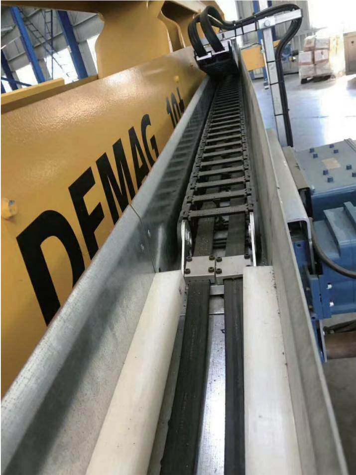
E3200.150.125.BK is used for small European style crane trolley sliding application, with a Travel length of 24 meters.
