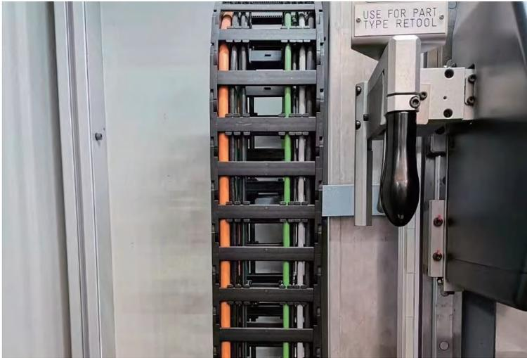
YFM3500.075.150.BK and other accessories are used for vertical standing applications of CNC machine tools
