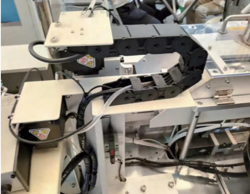
The application of ZFG1801 series energy chain in small automation equipment.
