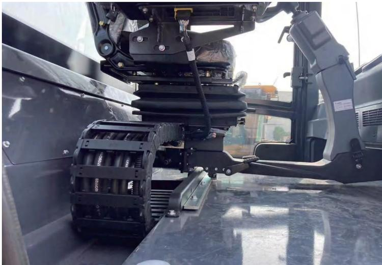
YFM3500.125.150.BK and other accessories are used for side-mounted movement applications on road machinery control consoles
