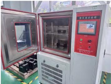
• High and Low Temperature Test Chamber
