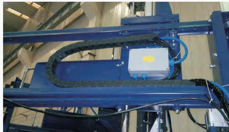
ZF1800 series is used for automated electronic equipment
