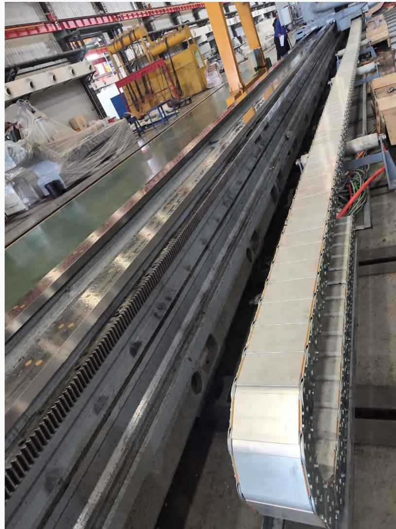
Application of ZF-TL125 in the long axis of heavy duty machine tool
