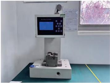
• Pendulum Impact Testing Machine
